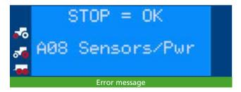
After rectifying the error, to resume full use of the central tire inflation system, it is necessary to switch it off and on again. To acknowledge the error, the operating console must be switched off and on again using the toggle switch.
