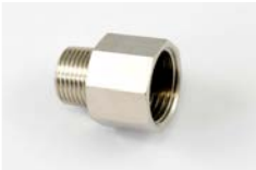
PTG-X-861-020 Reducer fitting 3/8" male to 1/2" female
