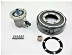
PTG-X-121-008 Rotary union kit RDS/GW 2L for ADR axle, AF155
