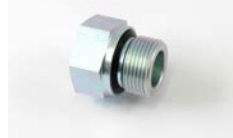
PTG-X-862-010 Reducer connector M22 x 1.5 male - 1/2" female
